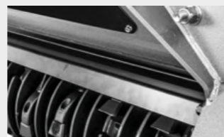
Dedicated rear hood (deflector) controls mulched material output for greater safety
