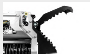
Excavator stand and hydraulic thumb useful in moving material to be mulched
